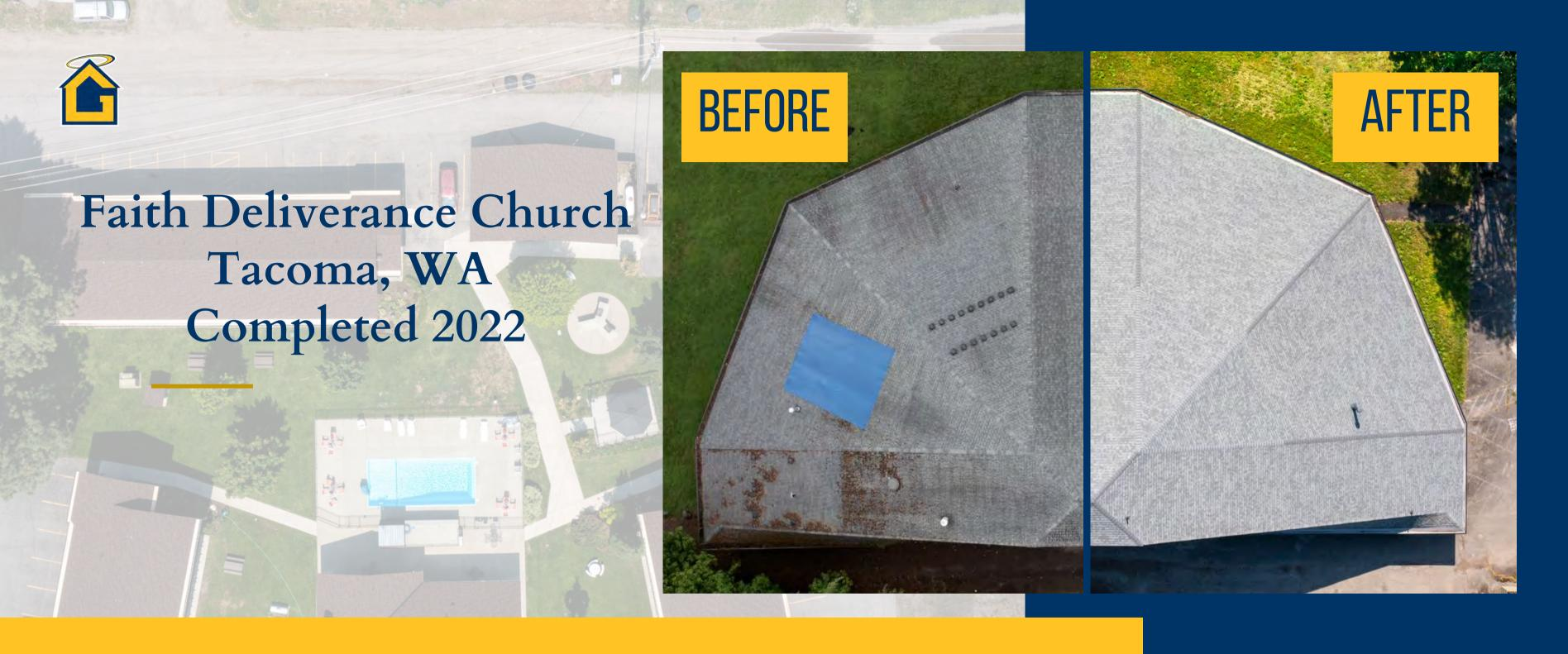
5000 Sq. Feet Church Remove existing Asphalt Shingles, Replace any Rotten Decking, and Install Owens Corning Oakridge Shingles
